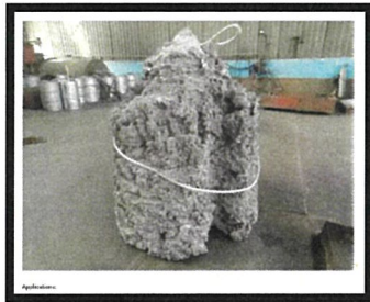
Typical sponge mass after crucible push-out
